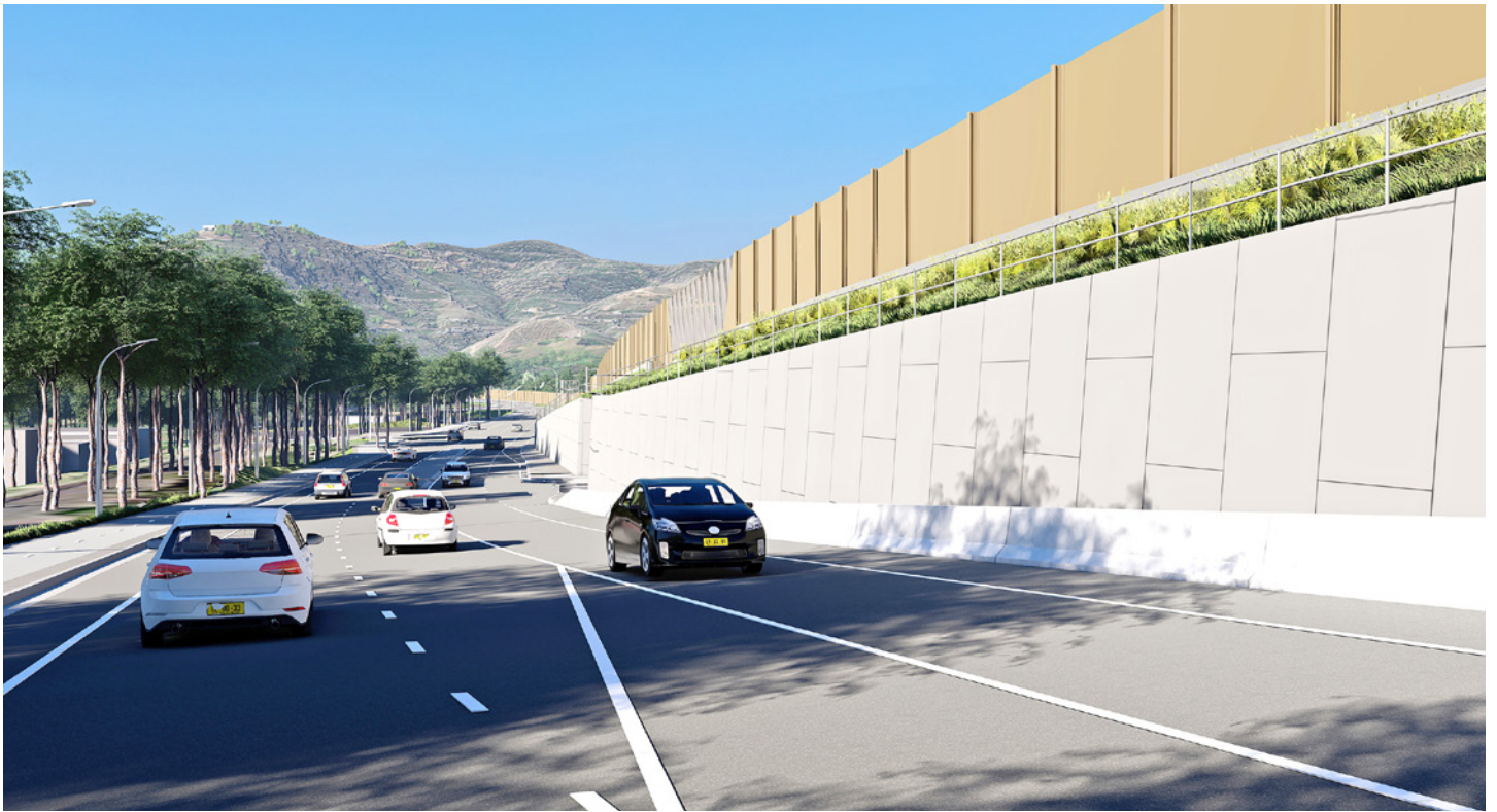
Artist impression of the retaining wall connecting to the Old Coast Road underpass
