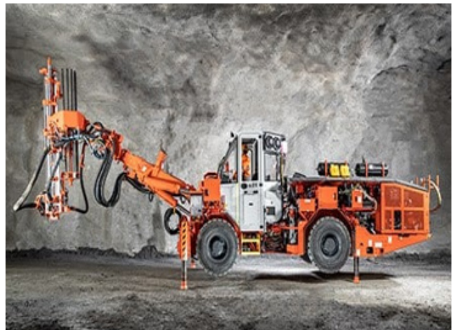
Large bolts and steel arches are installed into the walls and ceiling to support and stabilise the tunnel tube
