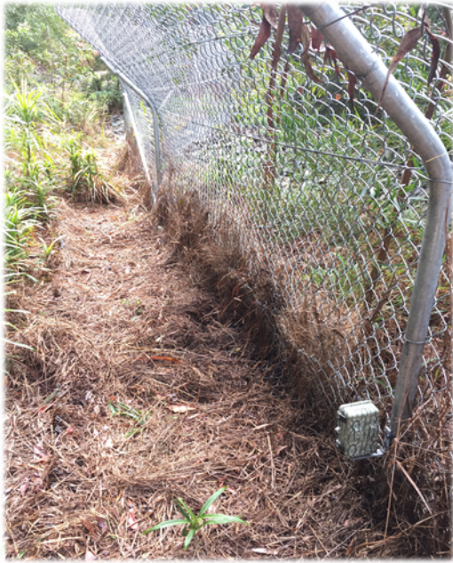
Plate 3: Typical exclusion fence camera set up. It shows a Scoutgaurd KG680V camera attached to a steel bracket which is fixed to a fence post.
