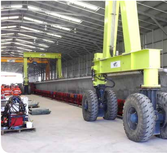
Using straddle carriers to remove the pre-cast girder from the formwork
