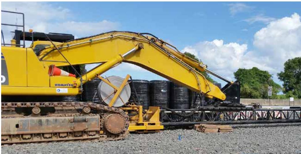
Wick rig arrives to site to start installing wick drains
