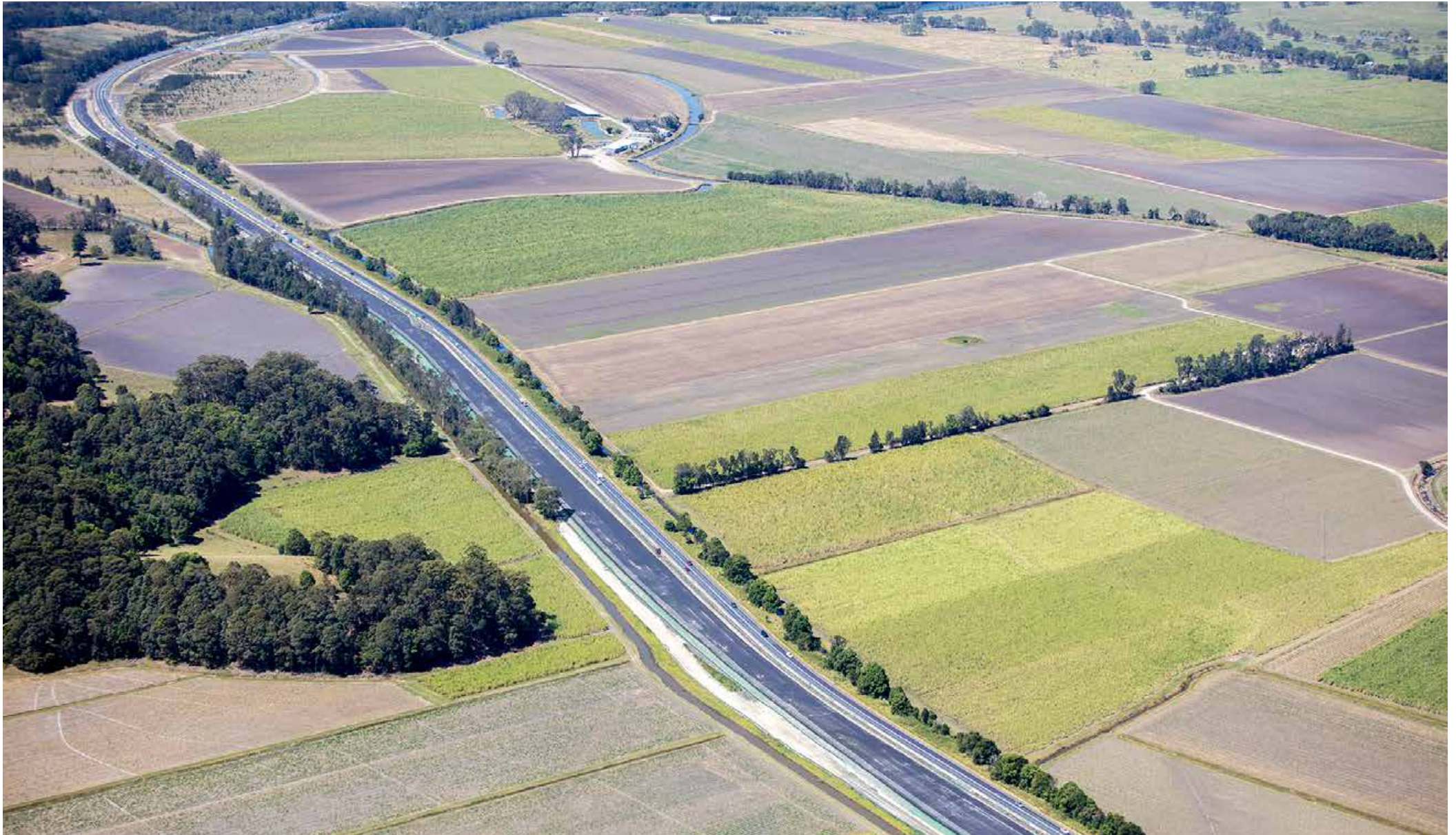
Aerial photo of new northbound carriageway undergoing soft soil settlement at Pimlico
