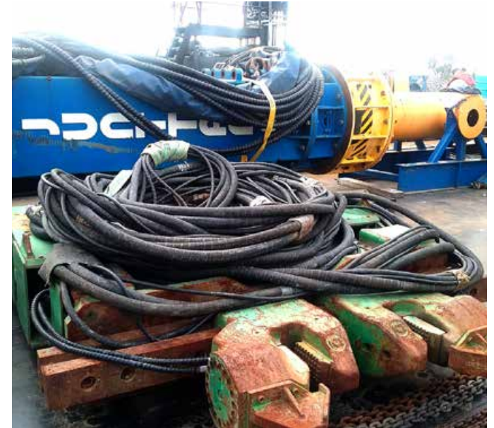
Vibration hammer for jetty piling
