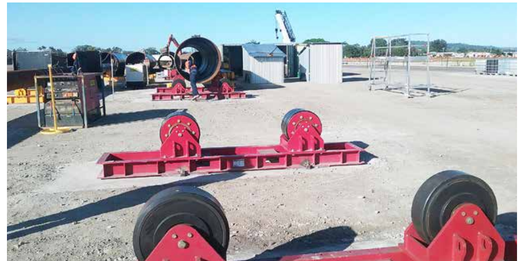
Pile casing rollers used to hold piles for welding
