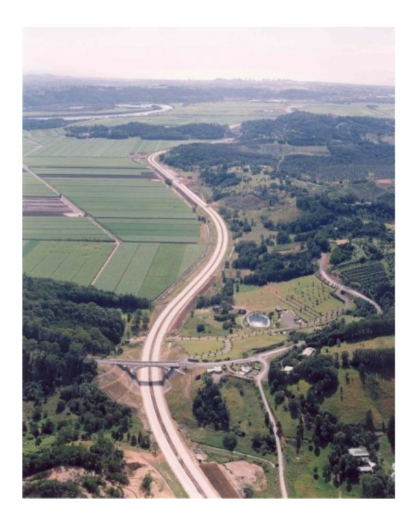
Example of how local access can be maintained in highway design
