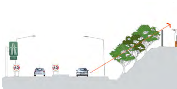
In a cutting the noise barrier located at top of a cutting is effective.
