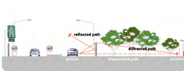
On level ground the noise barrier located close to source of sound is effective.
